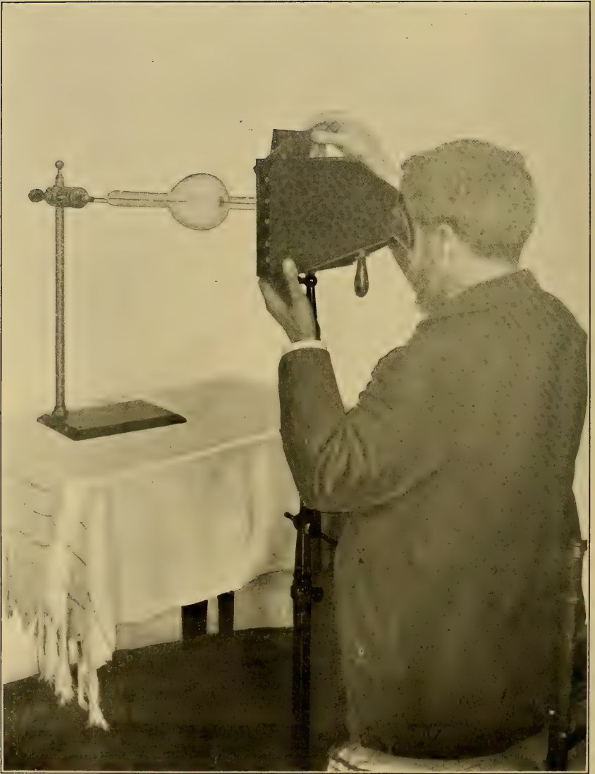
PLATE 46.—Author's X-Ray Gauge. This plate shows manner of shifting the shutters, one at a time, with the right hand while observing the effect of any degree of radiance upon the window and bars of the testing field. The operator sits in a chair with gauge and tube levelled to suit convenience. This is the only adequate and simple "meter" of X-radiance yet devised. By aid of the text and Instruction Plates any one can use it as taught. It is one of the prime necessities of scientific work with X-rays.
